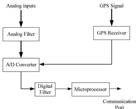
Fig. 1. The basic block diagram of PMU
