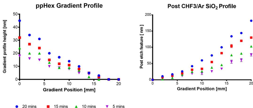
Fig. 2. The deposited ppHex gradient profiles (left), and their etched  $\text{SiO}_2$  profile correlations (right). The ppHex gradient masks were etched to ablation using  $\text{CHF}_3/\text{Ar}$  RIE, monitored by interferometry.
