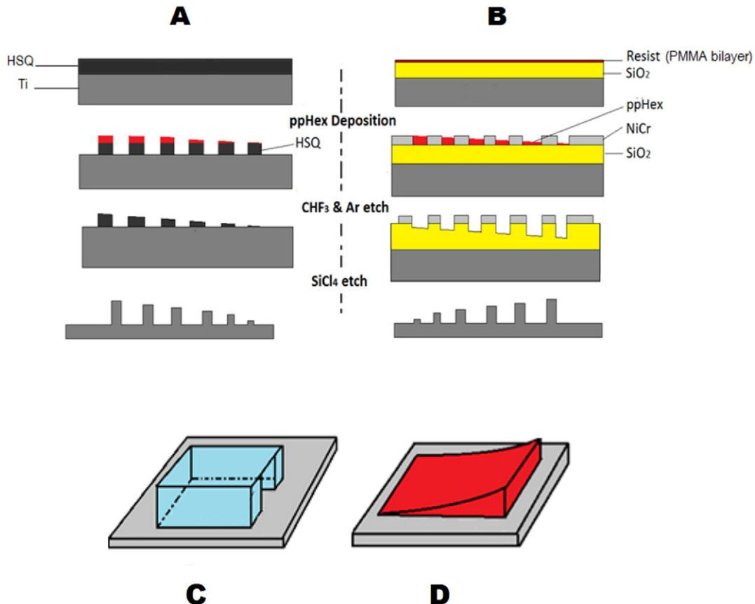
**Fig. 1.** (A) and (B) depict two routes to manufacture for the fabrication of pillar gradient arrays, made of titanium. (C) A diffusion limiting mask of dimensions: 20 × 15 × 8 mm, (D) a schematic of a ppHex gradient profile (mask removed) on a piece of titanium post deposition. Figure is not to scale.
