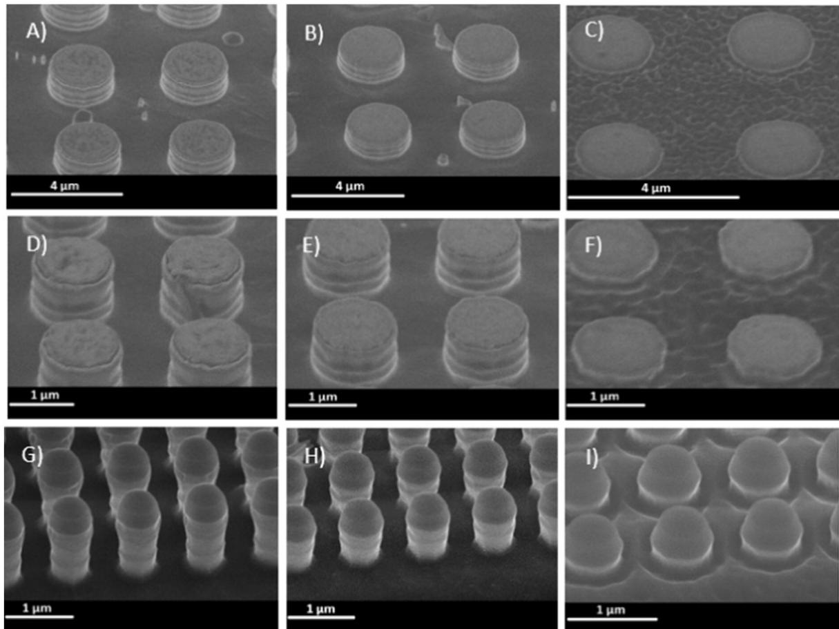
Fig. 4. Pillar topographies manufactured by  $\text{SiO}_2$  amplification (route B). (A–C, D–F) represent one sample featuring  $d = 2 \mu\text{m}$  and  $1 \mu\text{m}$  arrays respectively. G–I represents a separate sample,  $d = 500 \text{ nm}$ . Images in the left hand column were taken at (gradient position)  $X = 8 \text{ mm}$ , middle  $X = 4 \text{ mm}$ , right  $X = 0.2 \text{ mm}$ .
