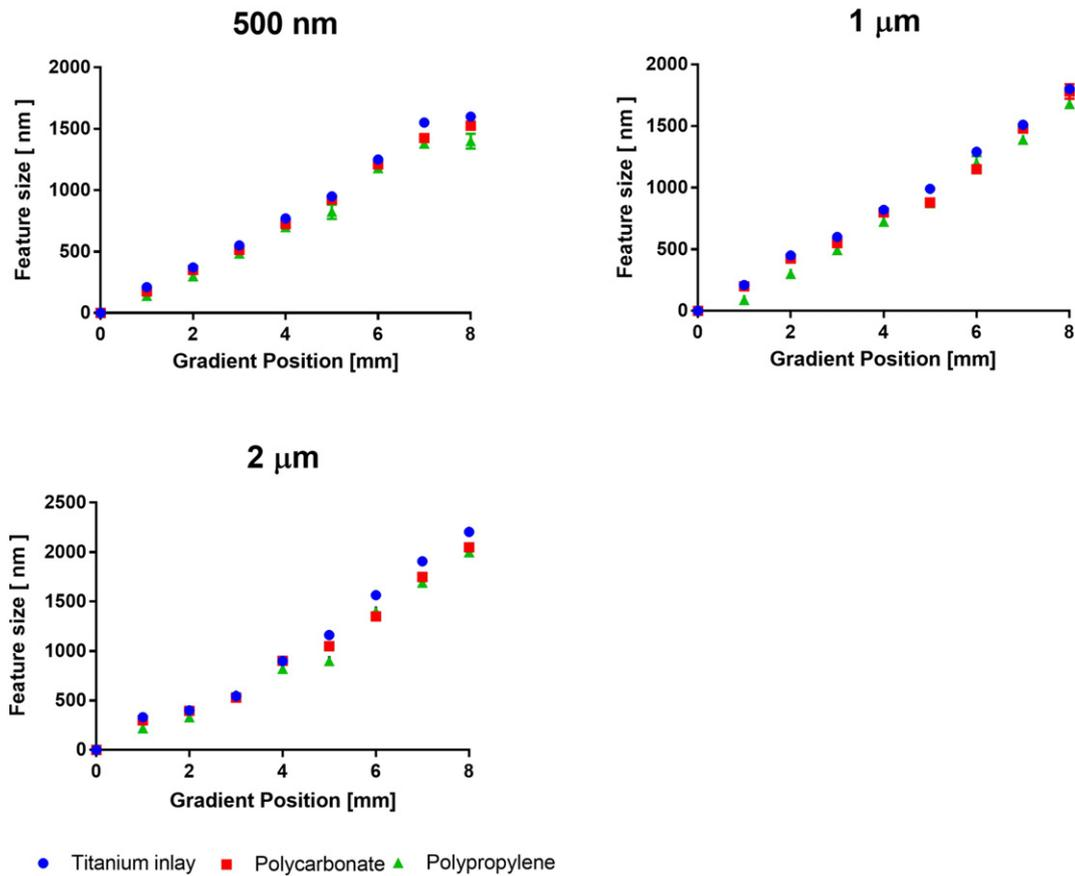
**Fig. 5.** The AFM measurement data above represents the Ti inlays manufactured by route B, i.e. pillar height. Also shown is the inverse profilometry data for polymer replicates (PC and PP), manufactured by injection moulding. RIE transfer dynamics explain the shortened gradient span from the original patterned array length.
