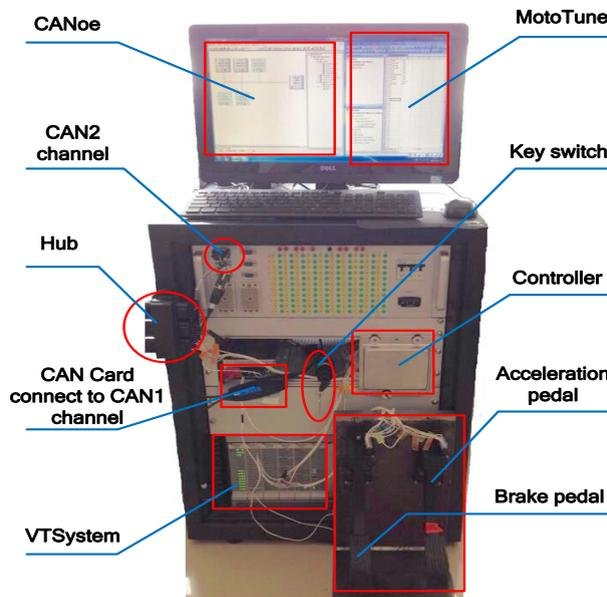
Fig.6. Hardware-in-loop simulation platform.
