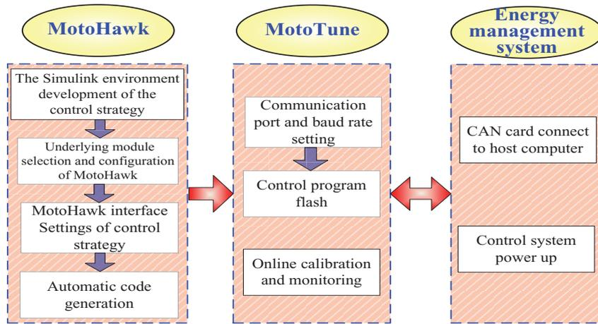
Fig.3. Control system development Based on MotoTron.
