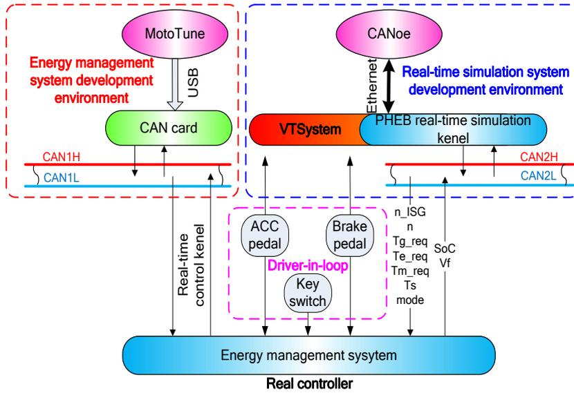
Fig.5. Structure of HIL simulation platform for receiving and sending signal.
