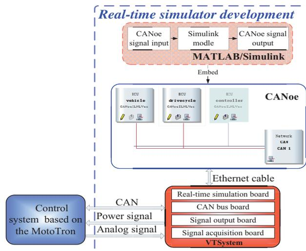
Fig.4. Real-time simulation system development based on VTSYSTEM.
