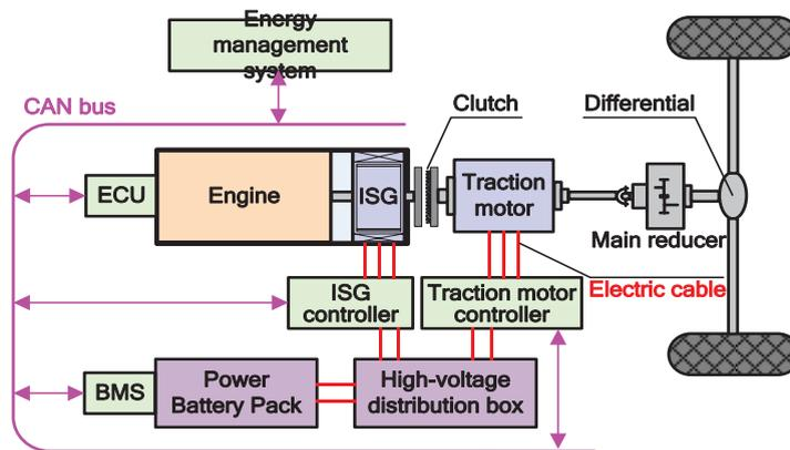
Fig.1. Powertrain architecture.
