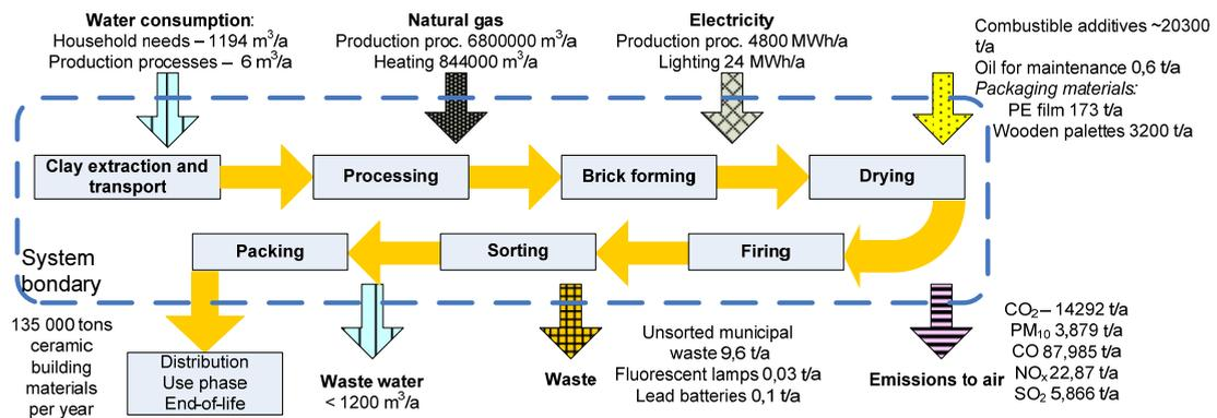
Fig. 1. Schematic presentation of the system boundary and the main inputs and outputs Life cycle impact assessment methodology and types of impacts
