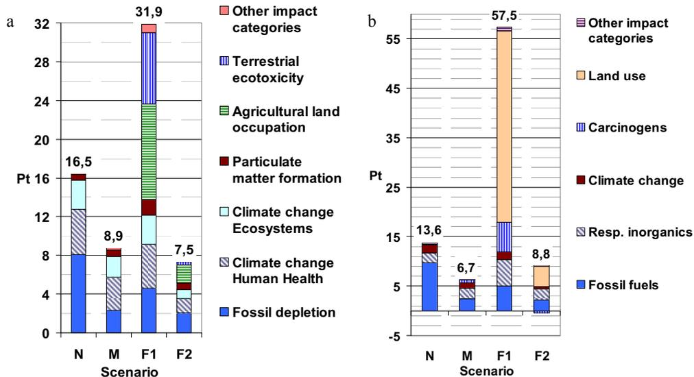
Fig. 2. Cumulated single score results of environmental impact per functional unit obtained using (a) *ReCiPe* and (b) *EcoIndicator’99* impact assessment method for the considered alternatives of the firing fuel. “N” – natural gas; “M” – bio-methane; “F1” – 1<sup>st</sup> generation bio-fuel; “F2” – 2<sup>nd</sup> generation bio-fuel
