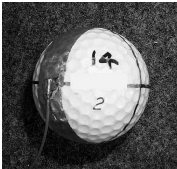
Figure 2 Wire soldered to a small patch of tape, with a conductive adhesive backing, attached to the surface of the conductive covering.
