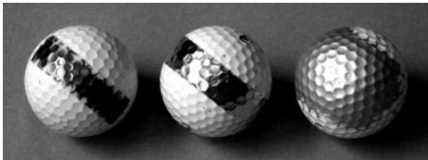
Figure 1 Three different techniques for applying a conductive coating to a golf ball: from left to right, embedded copper strip, aluminium foil and silver conductive paint.
