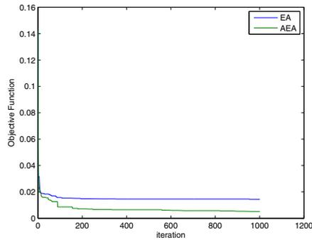
Fig. 3. Voltage deviation in the evolutionary process for EA and AEA in IEEE 14 busbar system
