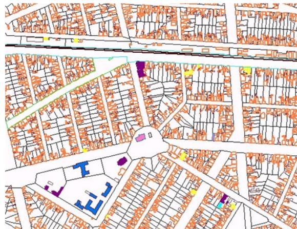
Figure 4. Generation using GIS software of the functionality classification (commercial, industrial, residential) of each building in an area situated in the city centre of Oradea
