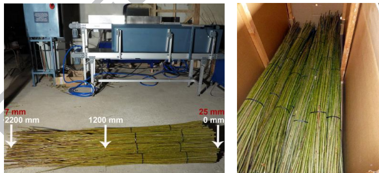
Figure 7. Cut, sorted and bundled harvested material using the proposed prototype
