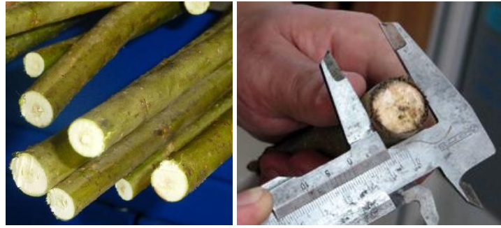
Figure 8. Cutting quality on willow (left) and poplar (right) rods
